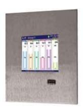
**Panel mount MultiCon ATG-500** is featured by a shallow casing – only 50 mm! All connectors are introduced on side walls of the device as in a typical panel computer. As the number of measurement inputs and outputs is limited, this design in intended mainly for systems with a small number of signals or systems which include other measurement systems with Modbus RTU interface. An Ethernet interface is also available to upgrade every MultiCon control's application easily.
